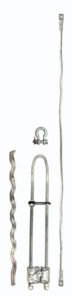
The Fiberlign Deadend is designed to terminate Optical Ground Wire (OPGW) while minimising any compression stresses that may be transferred to the core or optical elements within. The combination of retaining rods, wedge and housing distribute axial and compressive loading over a large area of the OPGW cable. Left-hand or right-hand lay style is provided to suit left-hand or right-hand lay OPGW respectively.
